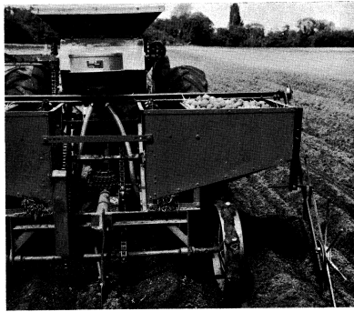
Fig. 1. Massey-Ferguson two-row automatic potato planter fitted with a Horsine Farmery granule applicator, planting an insecticide trial on the property of T. R. Mundy, Coult's Island, Canterbury. The applicator is in the centre (below the fertilizer bin) and the granules are metered by fluted rollers into the two tubes and down these into the furrow, falling alongside of and around the planted tuber. The fluted rollers within the applicator are turned by a horizontal drive shaft and this is driven by the ground wheel on the right of the planter.
